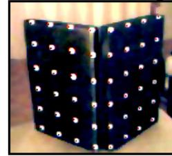
Figure 4 Calibration object
